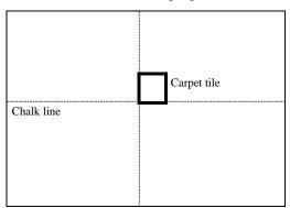
When laying the individual carpet tiles, care must be taken to ensure that none of the pile ends are squashed. Carpet tiles must be laid so that they fit together precisely.
